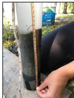
Figure 4. The longest sediment core retrieved from Pine Lake 2 was 21 cm long.
