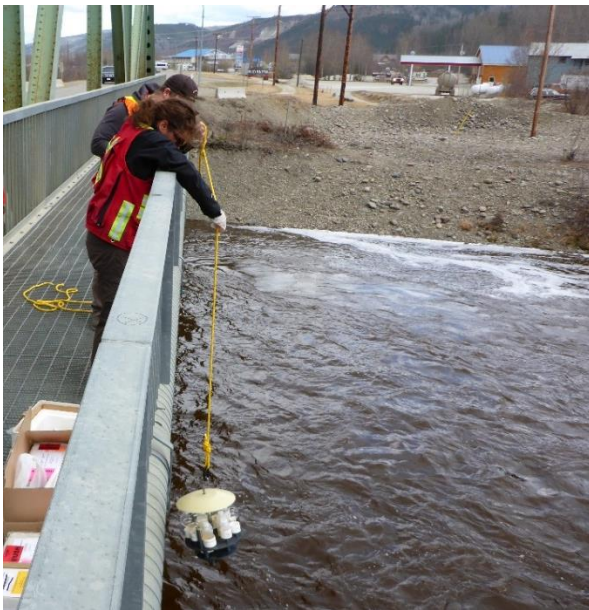
Water quality sampling at the Klondike Highway Bridge
