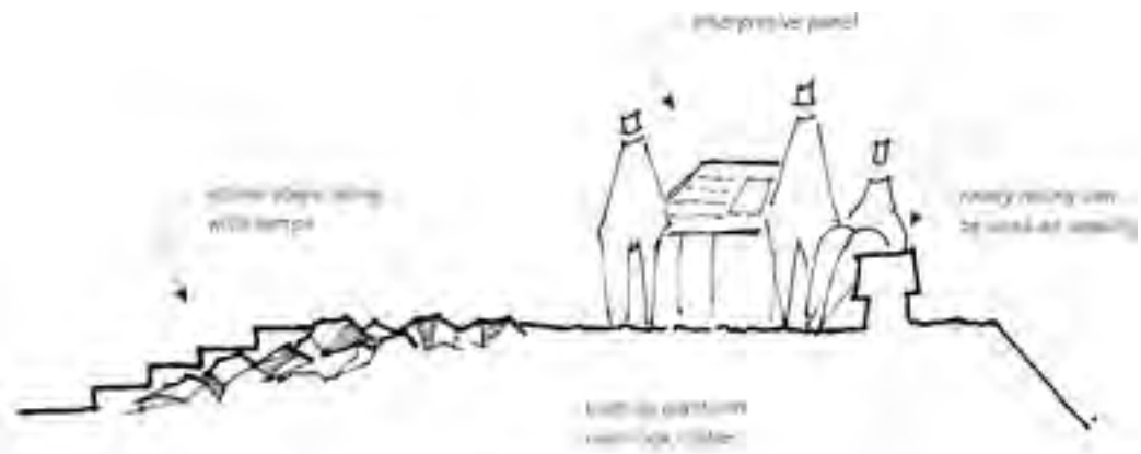
Profile of Viewing Platform
