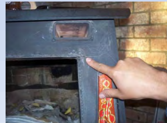
Cracked wood stove
