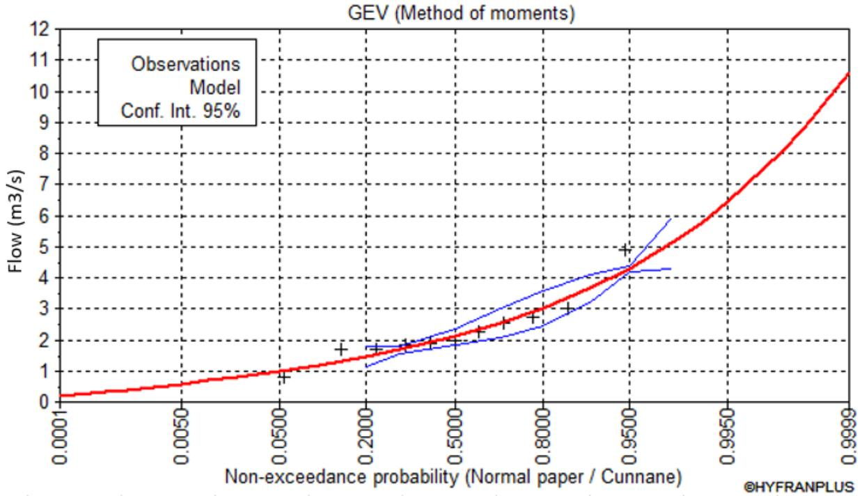
Figure 4.10. GEV Fitting for Station 09AA011
