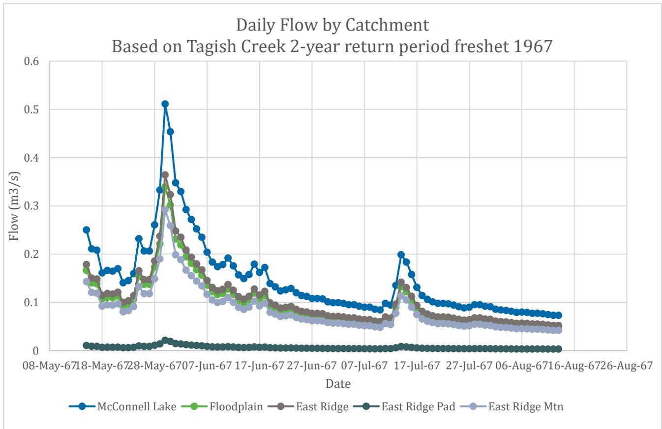
Figure 4.18. Hydrograph applied to Project area based on Tagish Creek 1967 2-year return period freshet.
