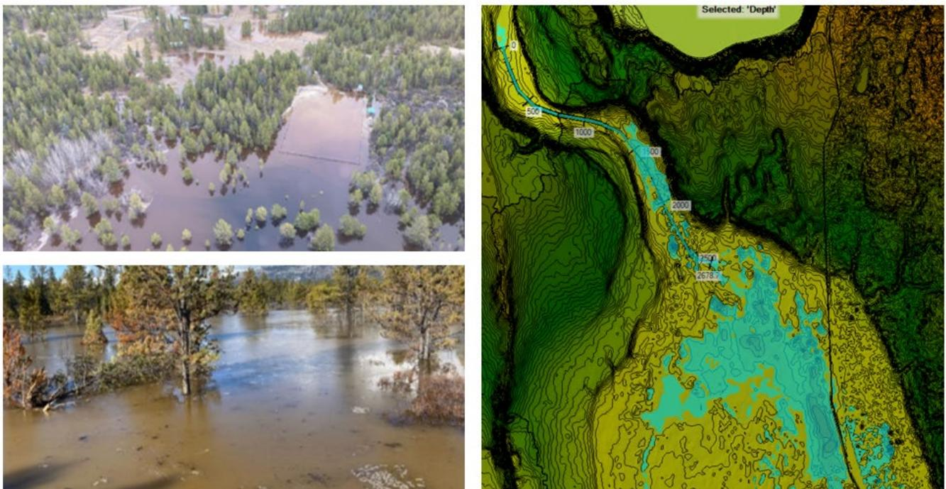
Figure 5.6: Comparison of modelled flood extents with diversion channel and field photos
