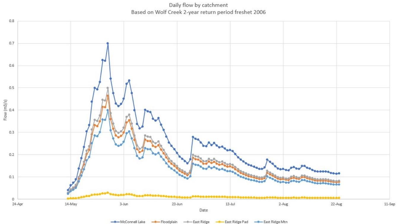
**Figure 4.12. Hydrograph applied to Project area based on Wolf Creek 2006 2-year return period freshet.**
