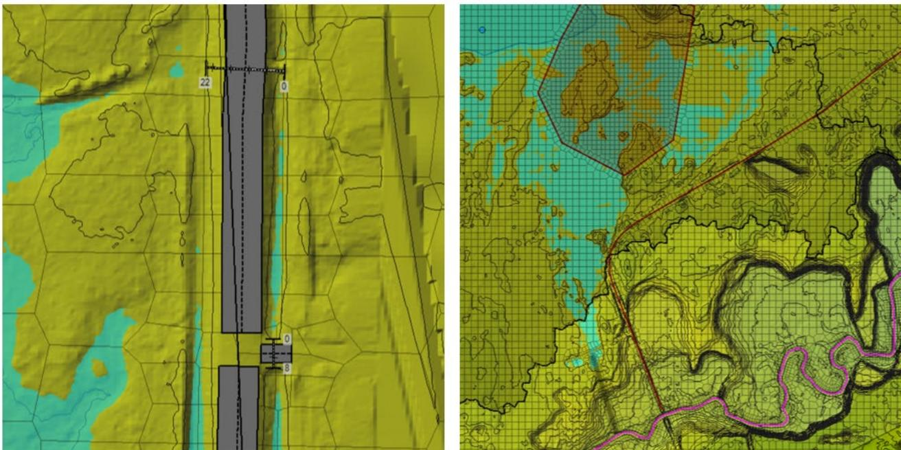
**Figure 4.3. Example Computation Mesh with a Refined Channel and Break Lines for Embankments**
