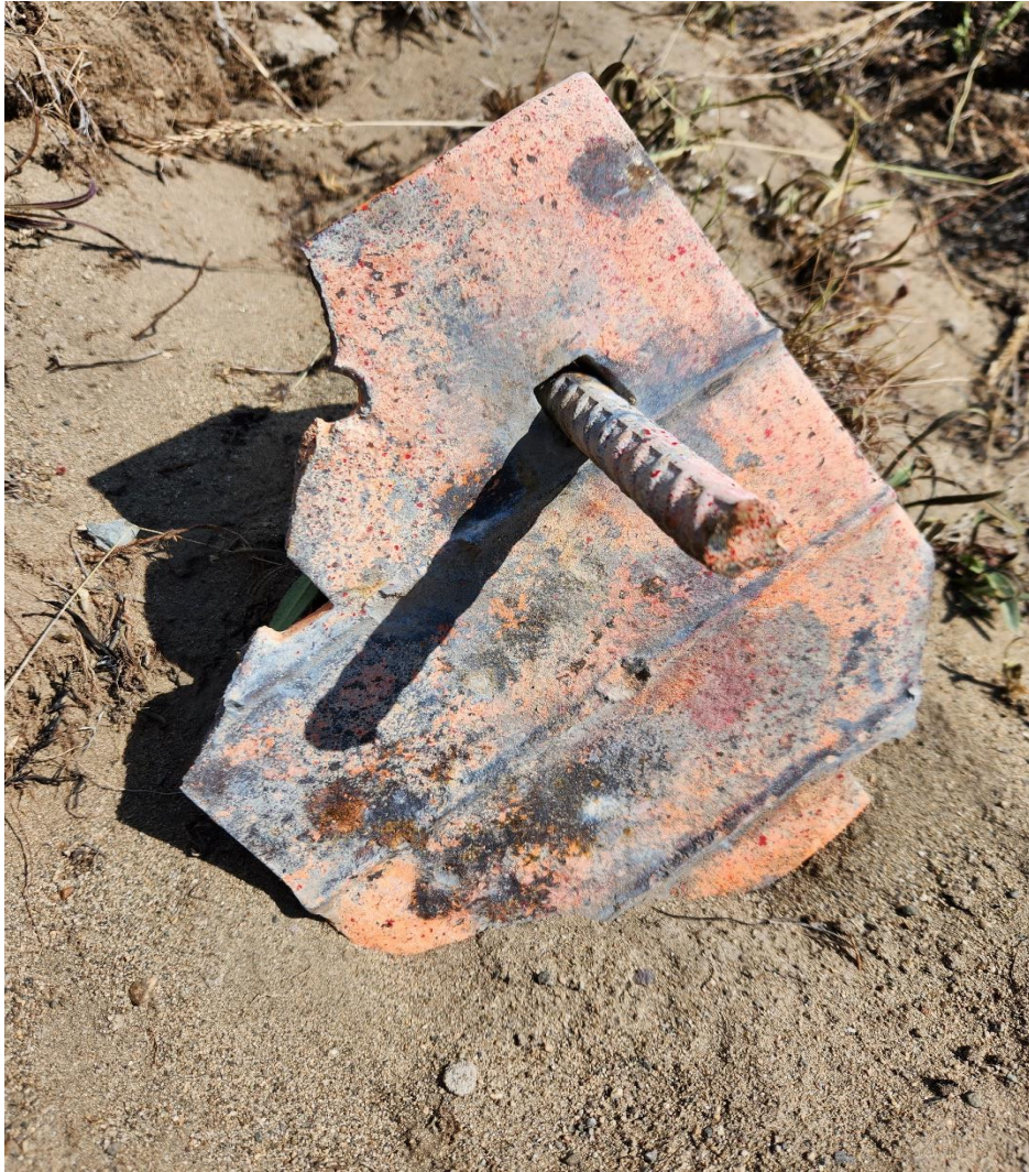
Figure 10: Iron target was secured to the slope with a single piece of rebar.
