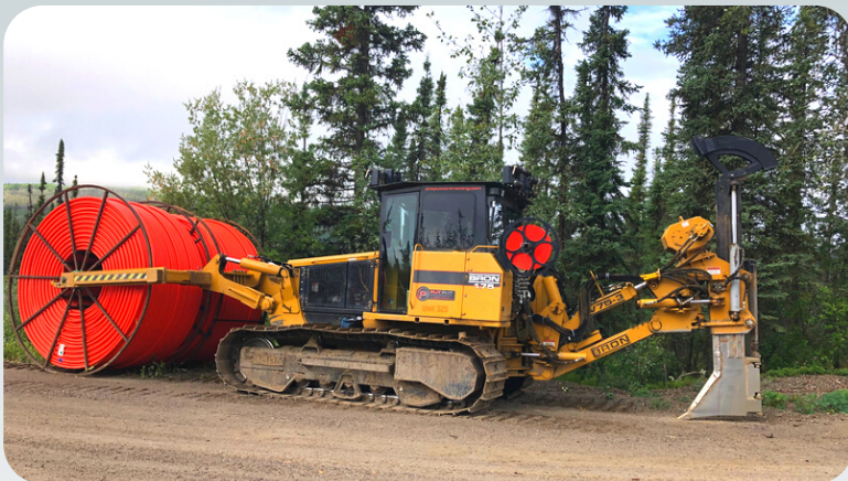
The plow cat, equipped with and ready to install cable conduit.
