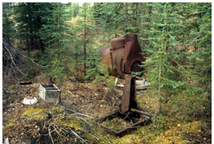
Boiler and steam points at a historic placer mining camp.
