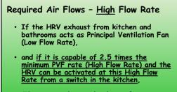
• Then no supplemental exhaust fans are required in the kitchen or bathrooms, i.e. the HRV can be the only required ventilation device in the home.
