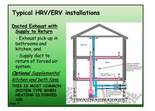
Canadian Prescriptive Codes (9.32) and Performance Standard (CAN/CSA-F326) both require a <u>High Airflow</u> and a <u>Low Airflow</u> Rate.
